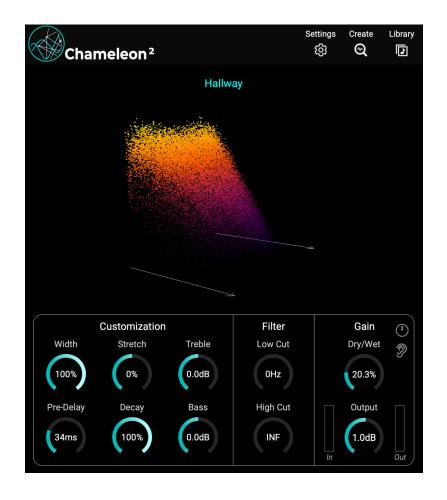
Chameleon is an intelligent reverb plugin which learns and imitates the room reverb of any source recording. After analysing a few seconds of audio, a reverb profile is built which exactly models the original room conditions and which can then be applied to match a dry studio recording. The ideal time-saving tool for ADR oder foley matching.
