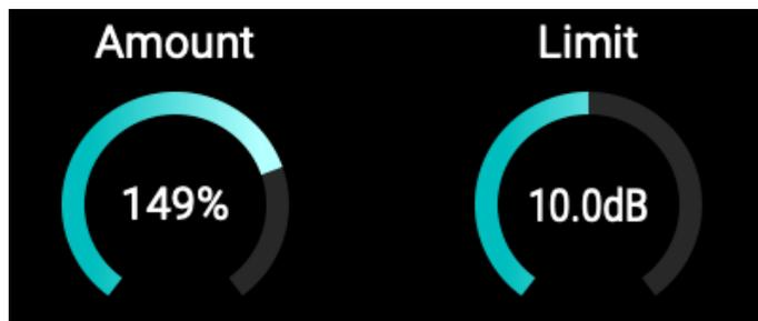
The Amount parameter defines how much of the automatically estimated gain correction should be applied to the signal. It also allows you to apply more gain than estimated by turning the control above 100%. Set to 0% no processing will happen at all.
