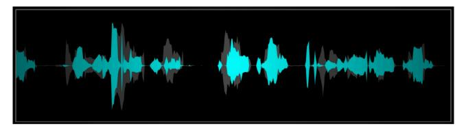
The upper visualisation shows the signal which is passing through the plugin either as waveform or spectrogram view. In waveform view the grey signal is the input signal while the coloured part is the signal after removing noise.
