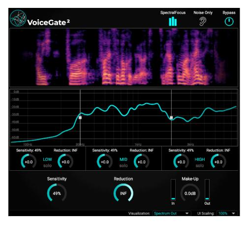
The crossover frequencies of the bands can be set by dragging the white squares of the band limit lines across the spectrum: By clicking on a solo button of a band you can solo listen to only this frequency region.
